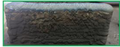
Fig. 4. Wall printed without defects using well-established parameters that have been controlled during the deposition.
