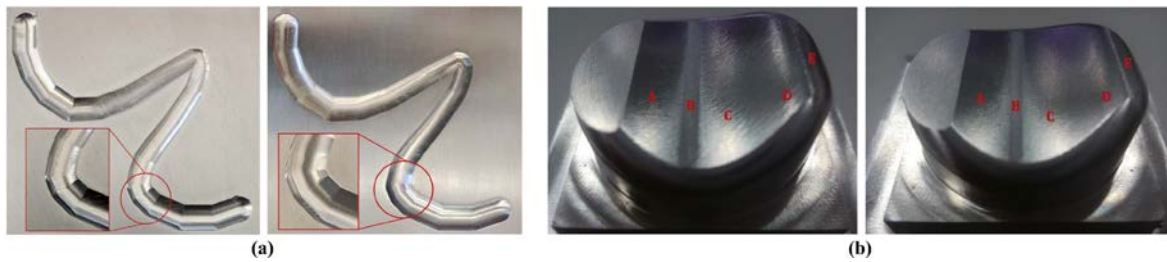
Fig. 15. Surface finish after corner smoothing of five-axis linear tool path. (a) Fan-shaped tool path after real machining using different corner smoothing methods, which the left figure uses the traditional G01 tool path and the right figure uses the corner smoothing method in Ref. 51; (b) Parts after real machining using different corner smoothing methods, which the left figure uses the traditional corner smoothing method and the right figure uses the corner smoothing method proposed in Ref. 55.
